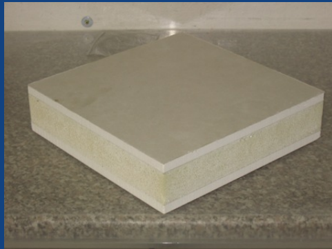
b) Precast systems based of anhydrite binder
